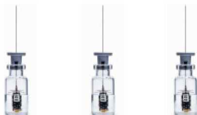
Fig. 1: Vial with wireless temperature sensor (Source of all figures and tables: iQ-mobil solutions GmbH).
