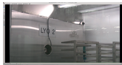
Fig. 15: TEMPRIS installation from outside through an unused flange.
