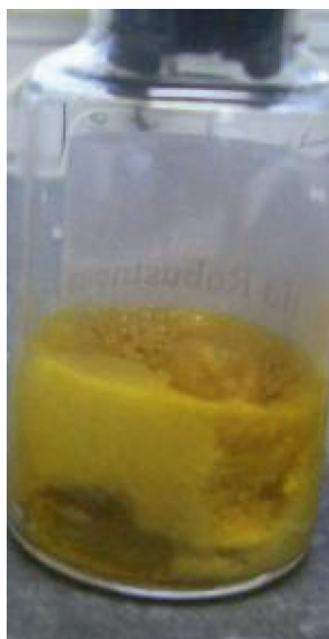
Fig. 8: Not acceptable meltback cake.
